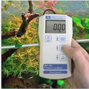
Turn the meter on by pressing the ON/OFF key. Press one of the three "Range keys" to select the proper scale according to the intensity of the light. 2000-19000 is recommended for measuring LUX in aquarium.
